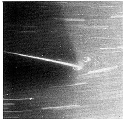
Fig. 5 Instantaneous flow visualization for k=1.2, U_\infty=20 cm/s, Re=2 \times 10^4, k=1.2, \alpha=-50 , downstroke
