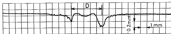
Fig. 6 Sectional curve of eroded specimen (apparatus 2 with nozzle holder A, HWBF, specimen B, P_u=9.9 MPa, P_d=0.14 MPa, L=10 mm, 15 hours)
