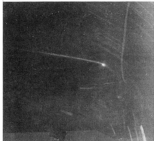
Fig. 8 Instantaneous flow visualization for k=3.9 , U_\infty = 10 cm/s, Re = 10^4 , \alpha = -0 deg downstroke
