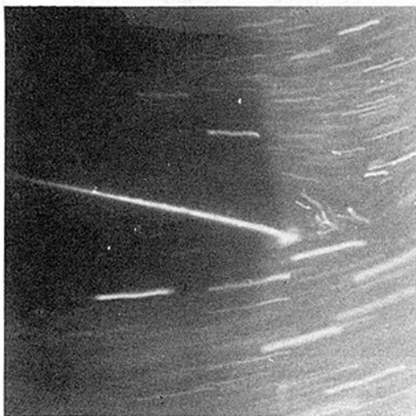
Fig. 7 Instantaneous flow visualization for k=2.4 , U_\infty = 10 cm/s, Re = 10^4 , \alpha = 0 deg upstroke
