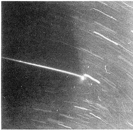
Fig. 6 Instantaneous flow visualization for k=2.4 , U_\infty = 10 cm/s, Re = 10^4 , \alpha = -0 upstroke
